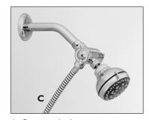
6. Connect the hexagon connector of the Hose (Part C) to the Diverter outlet.
